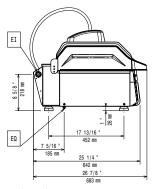
Electrical inlet (power) Electrical Outlet
